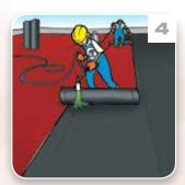
NOTE: If applied following the above recommendations, the resistance of the system (PLURA THERMO AD - PRATIKO P+V) to wind uplift will not be inferior to 7,0 kPa (700 kg/m²). (Official test report "Report BDA 0256-L-02")
