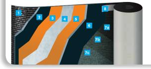
PLURA SELF-ADHESIVE has a continuous single strand composite woven non woven polyester reinforcement with high mechanical characteristics.
