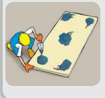
It is important that the application takes place at ambient temperature not lower than  $+ 5 \,^{\circ}$ C.
